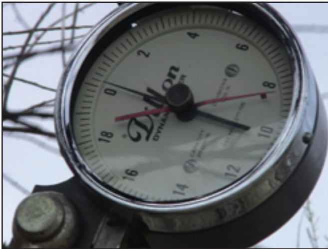
Figure 2—A Dillon 20,000-pound dynamometer used to determine how much force was needed to pull tamarisk.
