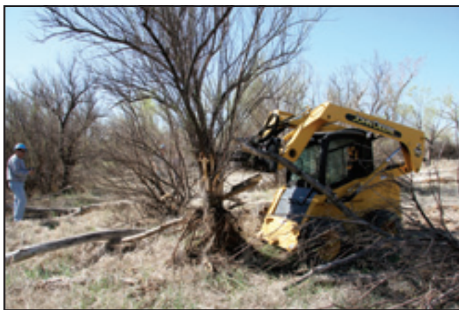
Figure 5—Tamarisk pulled up by the John Deere 260 skid steer loader. Note the size of the tamarisk's root.
