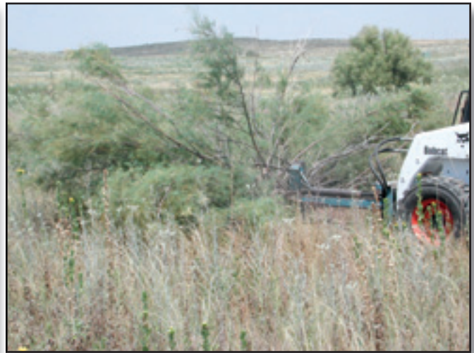
Figure 9c—The Bobcat brush saw being used to cut tamarisk.
