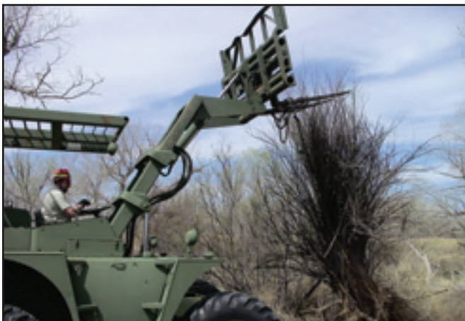
Figure 3a—A surplus military forklift designed for rough terrain was used to pull out tamarisk.
