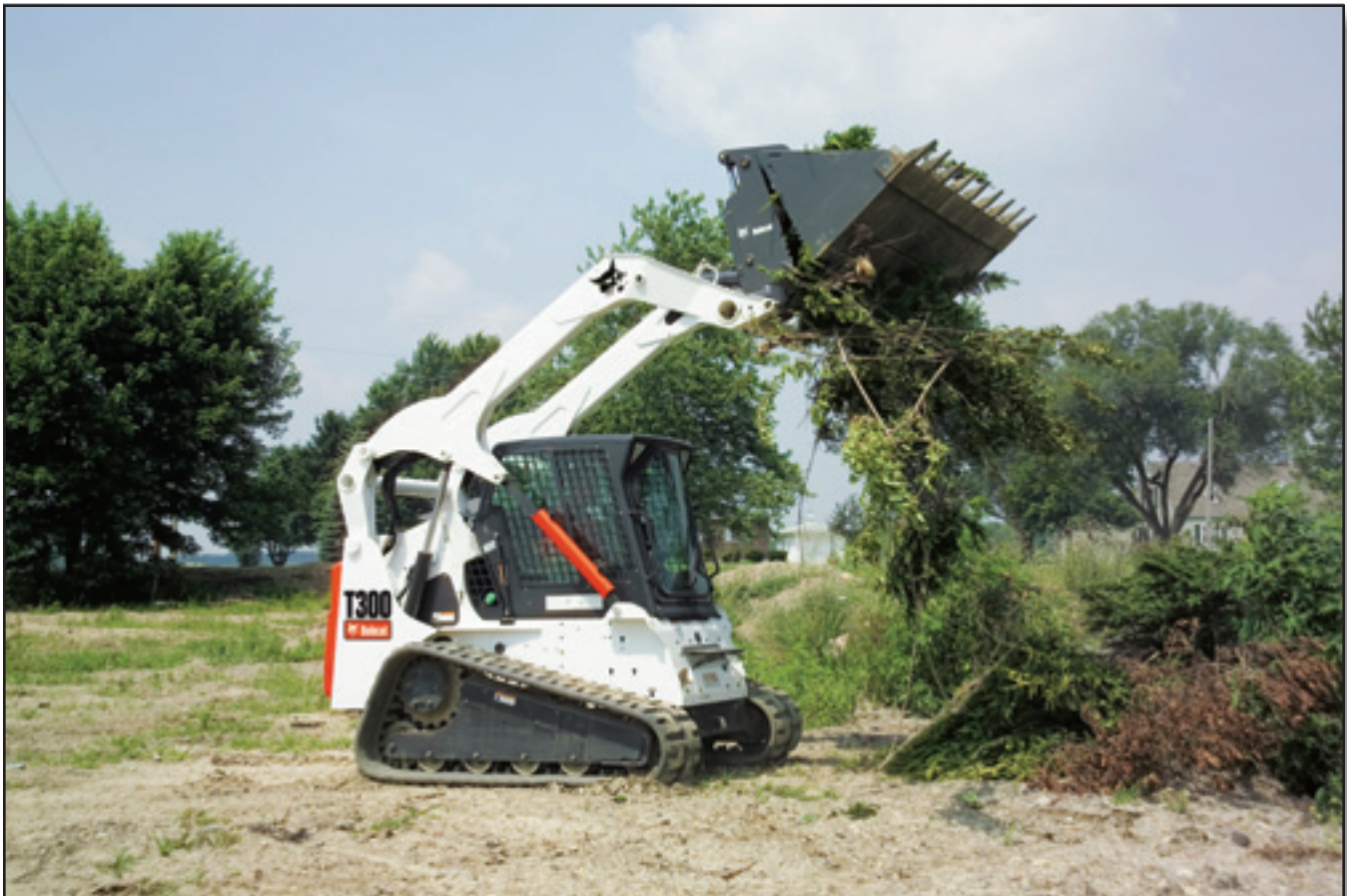
Figure 8—T300 Bobcat Compact Track Loader (Photo courtesy of Bobcat Co.). No photos with the JAWZ mounted on the T300 were available.
