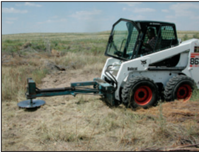
Figure 9a—A Bobcat brush saw mounted on a skid steer loader.
