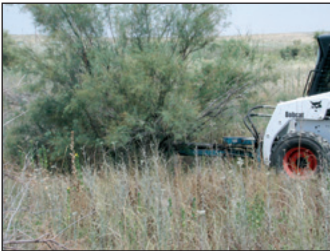
Figure 9b—The skid steer loader equipped with a Bobcat brush saw approaches a tamarisk plant.
