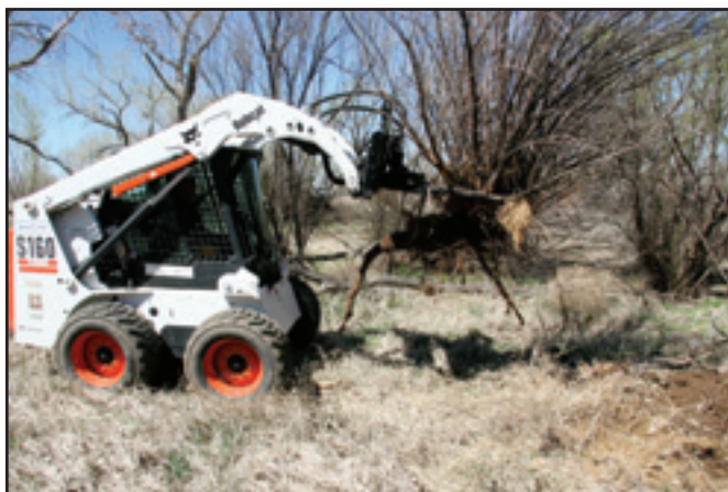
Figure 4—The Bobcat S160 skid steer loader.
