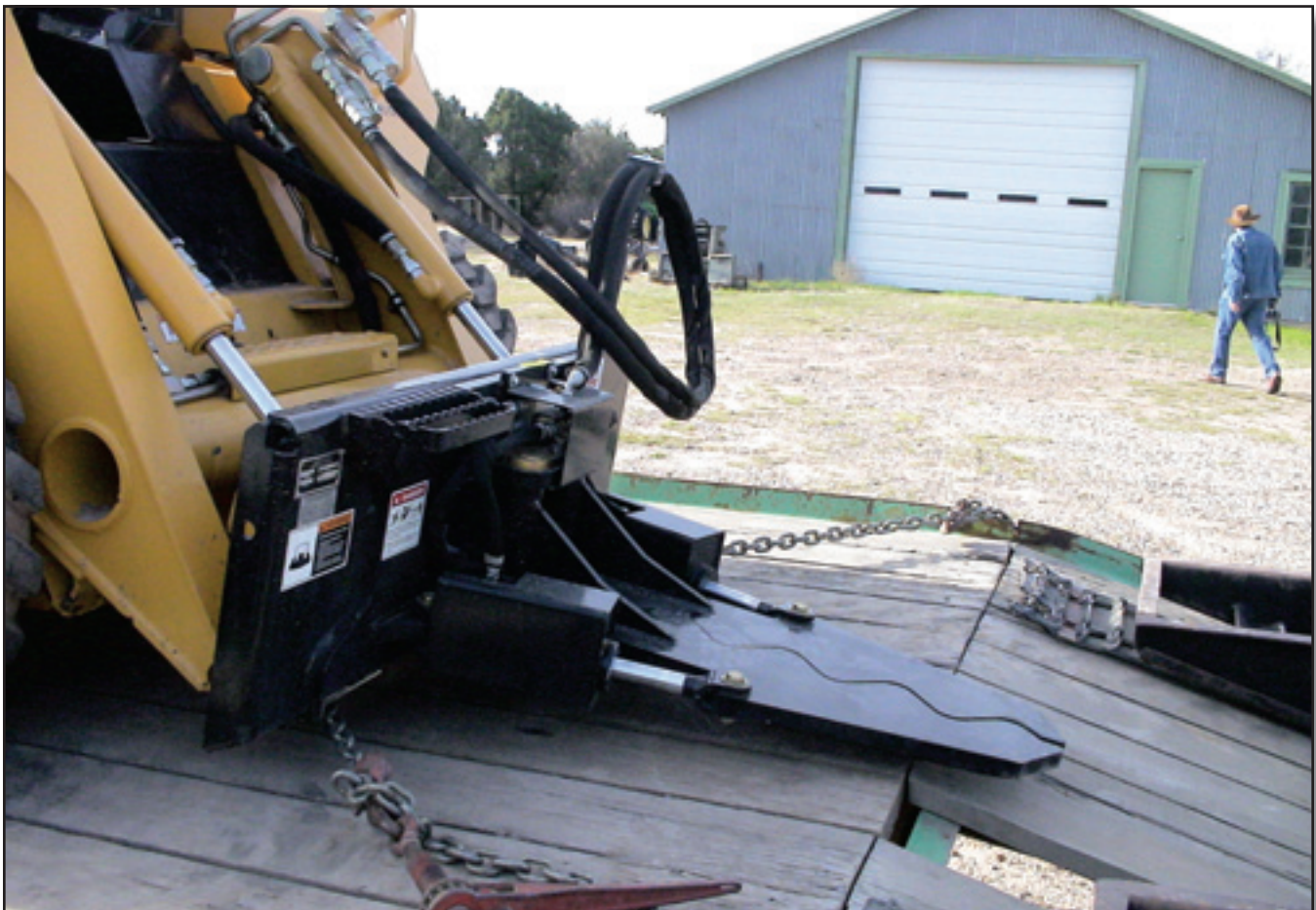
Figure 1—The Star Hill JAWZ attachment was used to pull tamarisk plants from the ground.
