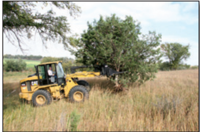
Figure 17a—Star Hill Super JAWZ on a Caterpillar 924 removing a tree (Photo courtesy of Starhill Solutions, Inc.).
