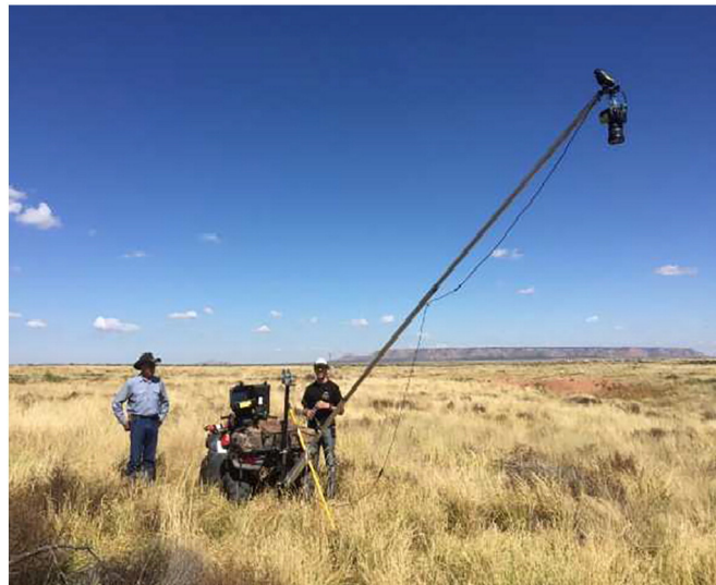
Figure 2. High-resolution camera and computer mounted on four-wheeler used for ground-based vertical photographs (GBVP).
