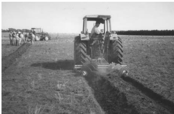
Merbein Plough (above) and Rippa Moulder (below) in action
