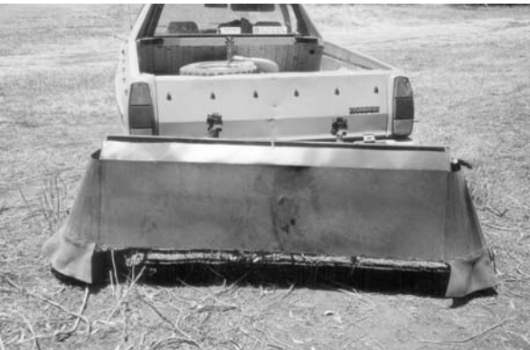
Handheld shielded spray applicator (above) and a shielded spray unit mounted on a utility
