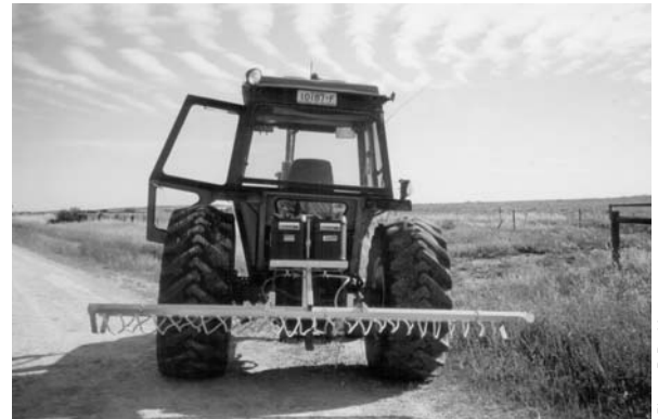
Rope Wick Applicator being used for selective weed control
