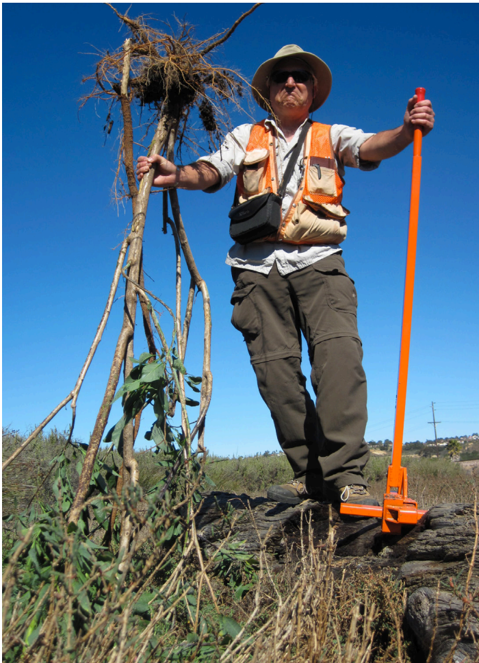
A weed wrench is a useful tool for mechanical removal of invasive plants. Photo: Doug Gibson, San Elijo Lagoon Conservancy
