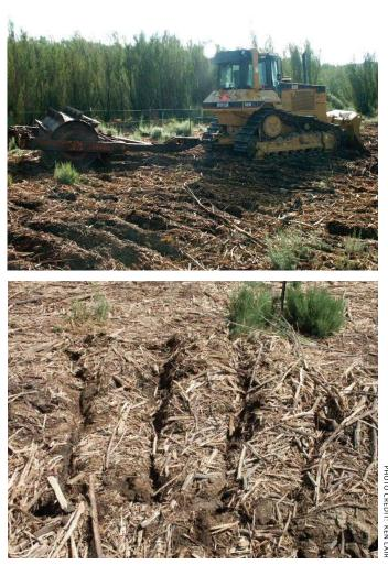
**FIGURE 19:** The roller chopper shown above has been used to create surface texture after tamarisk was cleared from a site.
