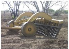
**Ripper/Deep Chisel Type Root Plow**
