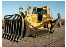
**Ripper/Deep Chisel Type Root Plow**
