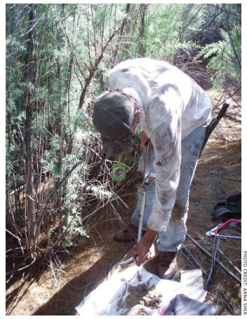
FIGURE 5: Soil sampling of the top foot of soil using a steel soil auger (also called a probe).
