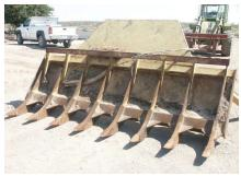
**Ripper/Deep Chisel Type Root Plow**
