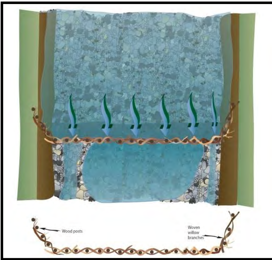
Figure 26: Diagram of a starter dam, showing design detail and the necessary material needed for construction. (top) side view (bottom) plan view.
