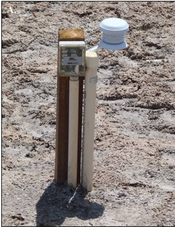
Figure 16. Remote weather stations installed on the burn revegetation demonstration studies, Cibola National Wildlife Refuge, Cibola, Arizona. A. HOBOT MicroStation™ installed on all three study sites, with sensors for air temperature and humidity at 60 cm height, and soil moisture and temperature at 15 cm soil depth. B. HOBOT Weather Station installed adjacent to Demonstration Study 1, with a full array of sensors as described in the narrative text.
