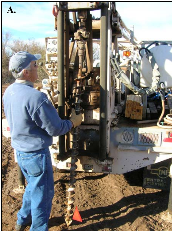
Figure 10. Drill rig used to auger holes at the study site (Image A), and backfilling of holes with zeolite (Image B).
