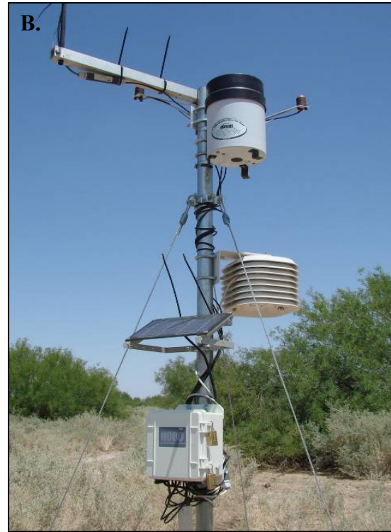
Figure 16. Remote weather stations installed on the burn revegetation demonstration studies, Cibola National Wildlife Refuge, Cibola, Arizona. A. HOBOT MicroStation™ installed on all three study sites, with sensors for air temperature and humidity at 60 cm height, and soil moisture and temperature at 15 cm soil depth. B. HOBOT Weather Station installed adjacent to Demonstration Study 1, with a full array of sensors as described in the narrative text.
