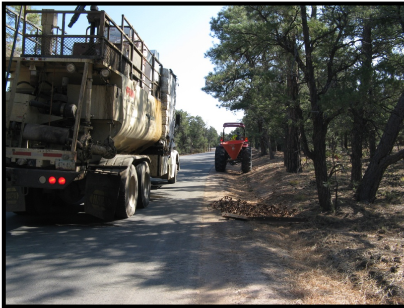
Tractor mounted broadcast seeder, backing up to a drag harrow, which is lying behind it. The hydromulcher is directly behind the tractor, waiting to spread hydromulch after the tractor operator spreads seed and incorporates it by scarification.
