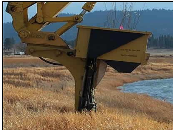
Figure 3.18 Rotary Stinger used for deep planting from Los Lunas Plant Materials Center.
