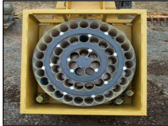
Figure 3.20 Plant container portion of Rotary Stinger.
