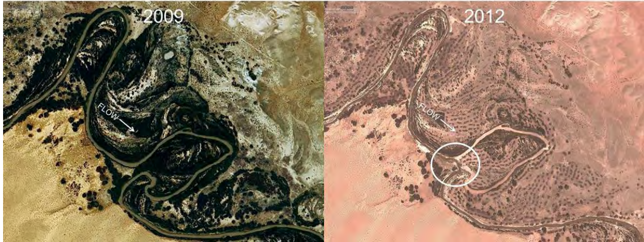
Figure 52. Aerial photographs of a reach of the San Rafael River taken in 2009 and 2012. Dots on the floodplain in the 2012 photo are piles of tamarisk that were removed by the UDWR in 2009-2010. In 2011 a large magnitude, long duration spring snowmelt flood occurred and caused a channel avulsion and meander cutoff event, seen in the circle on the 2012 photograph.
