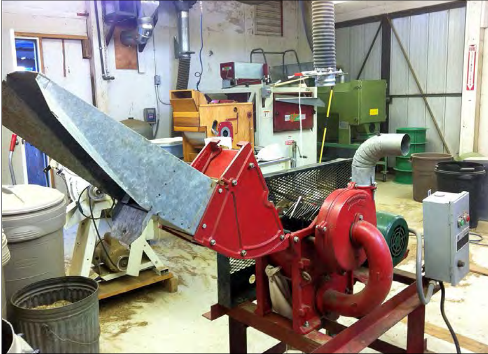
Hammermill. The chamber is in front of the grid. (Photo: Brianna Borders, The Xerces Society.)
