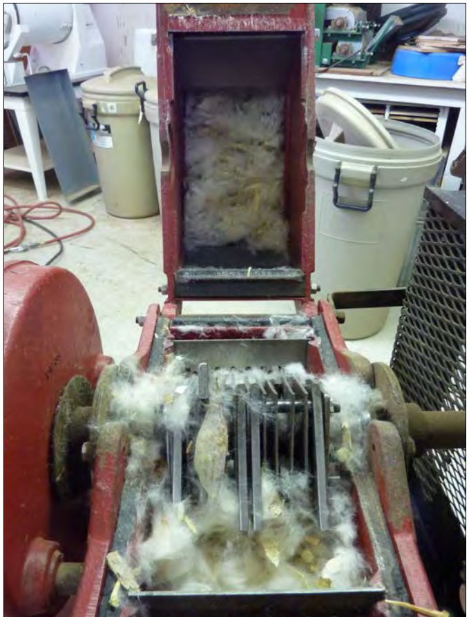
Partially processed showy milkweed pods in a hammermill chamber at the USDA-NRCS Plant Materials Center in Corvallis, Oregon. (Photo: Brianna Borders, The Xerces Society.)
