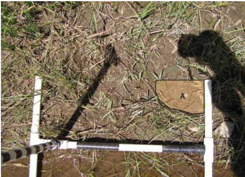
Figure A8. The greenline must have at least 25 percent cover and there are no patches of bare ground larger than 10 percent of the plot. Area "A" is at least 10 percent; therefore, the monitoring frame is not on the greenline.
