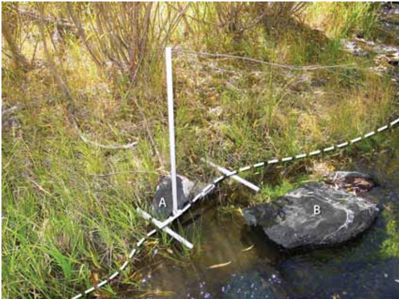
Figure A20. Rock "A" is embedded and above the scour line. Active erosion exists on the streambank side of rock "B," and it is below the scour line.
