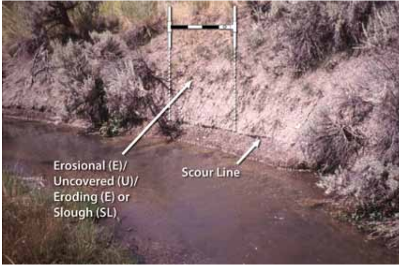
Figure E11. The streambank has an obvious scour line. The bank evaluated is above the scour line to the first bench and is recorded as erosional (E), uncovered (U), and eroding (E) or slough (SL).
