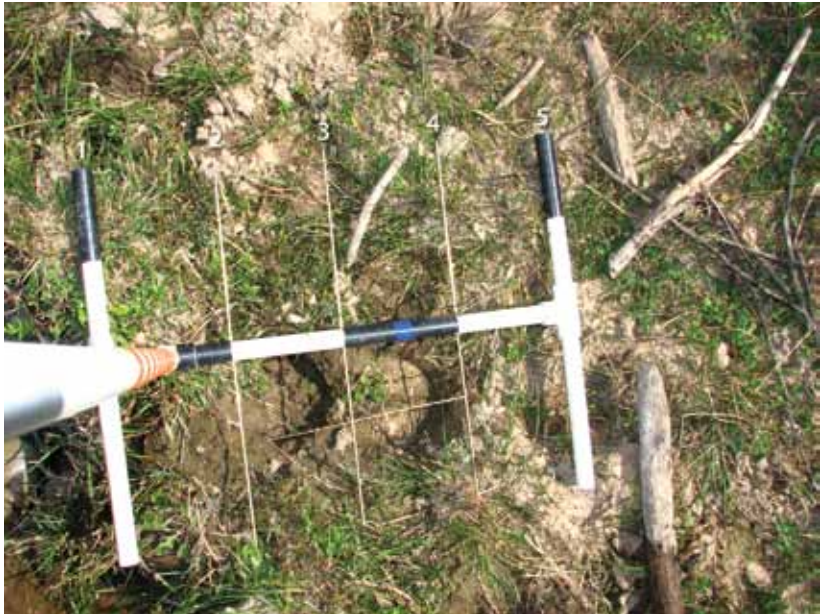
Figure D2. The monitoring frame is centered on the greenline and the number of lines (0 to 5) that intersect streambank alteration (trampling or shearing) is counted and recorded. Lines 1, 2, 3, 4, and 5 intersect streambank alteration. A "5" is recorded.
