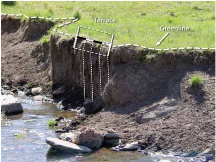
Figure D5. Trampling on the terrace is not recorded as streambank alteration. Alteration is only recorded if it occurs on the steep face of the bank. The lines are projected for the greenline down the bank, within the monitoring frame. In the example above, line 1, nearest the handle, does not intersect alteration. Lines 2 through 5 intersect shears so a “4” is recorded.
