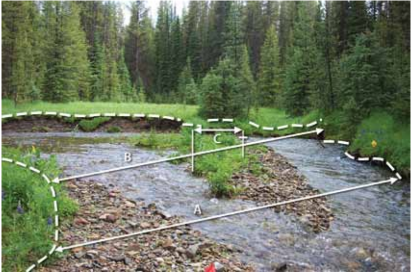
Figure G5. Line “A” is the total length of the GGW. The gravel bar has no vegetation. When the GGW crosses an island with at least 25 percent cover, the nonvegetated portion is calculated (total length of line “B” – line “C”) to determine the nonvegetated portion of the two channels. Photo - PIBO, U.S. Forest Service.
