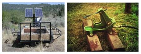
Figure 10. Creating upland water sources with a mobile solar powered pump (left) and nose pump mounted on railroad ties (right).
