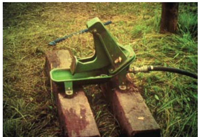
Figure 22. Pasture nose pump mounted on railroad ties. (Photo by S. Wyman, NRST.)
