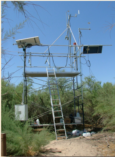
Tower with micrometeorological and eddy covariance sensors for measuring evapotranspiration of riparian vegetation along the lower Colorado River, California.
