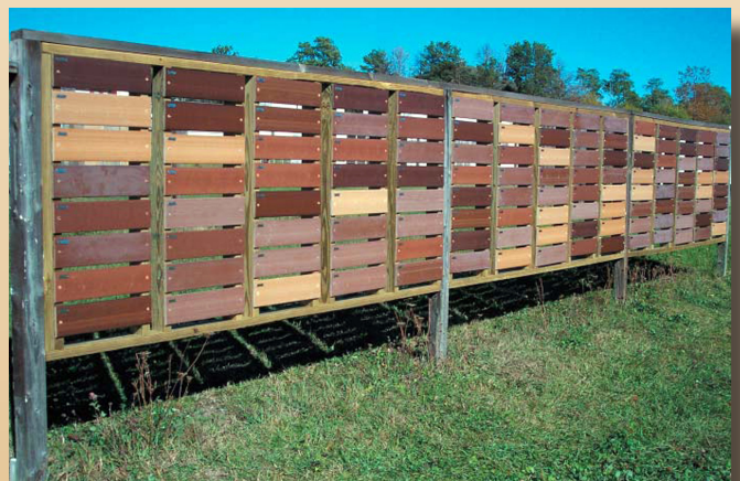
Natural weathering test rack with extruded composite boards manufactured from saltcedar-, juniper-, and pine-wood flours. Saltcedar boards are those with the darkest coloring. Photo: U.S. Forest Service.
