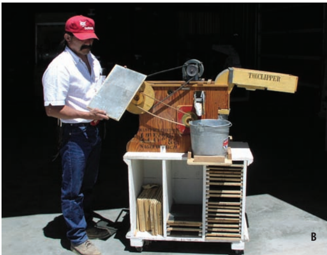
Figure 7.12 —Commercial seed cleaners such as (A) a hammermill or (B) clippers are useful for cleaning large lots of native seeds. Photos by J. Chris Hoag.
