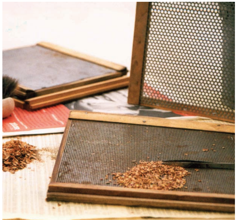
Figure 7.11 —Screens are used to separate large debris, seeds, and fine chaff from the seedlot and are available commercially in a wide range of screen holes sizes to complement any species. Photo by Tara Luna.
