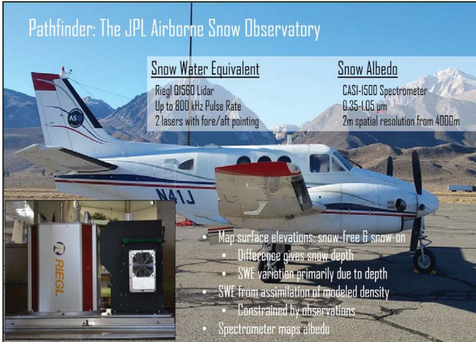
The Airborne Snow Observatory systems is being tested by the Jet Propulsion Lab as a new, improved way to measure snowpack in order to better predict runoff and streamflows.
