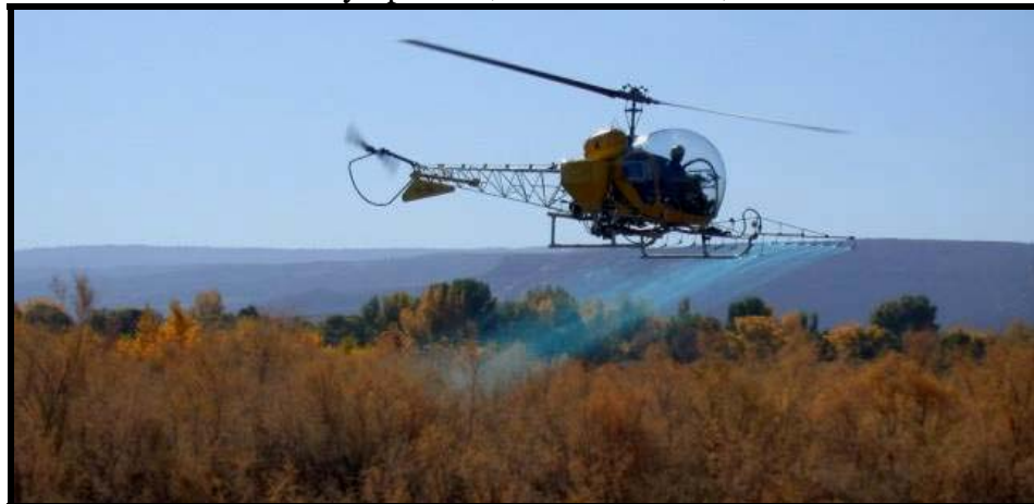
Figure 13: Aerial herbicide application technique being demonstrated with dyed water at 2003 Tamarisk Symposium, Grand Junction, Colorado
