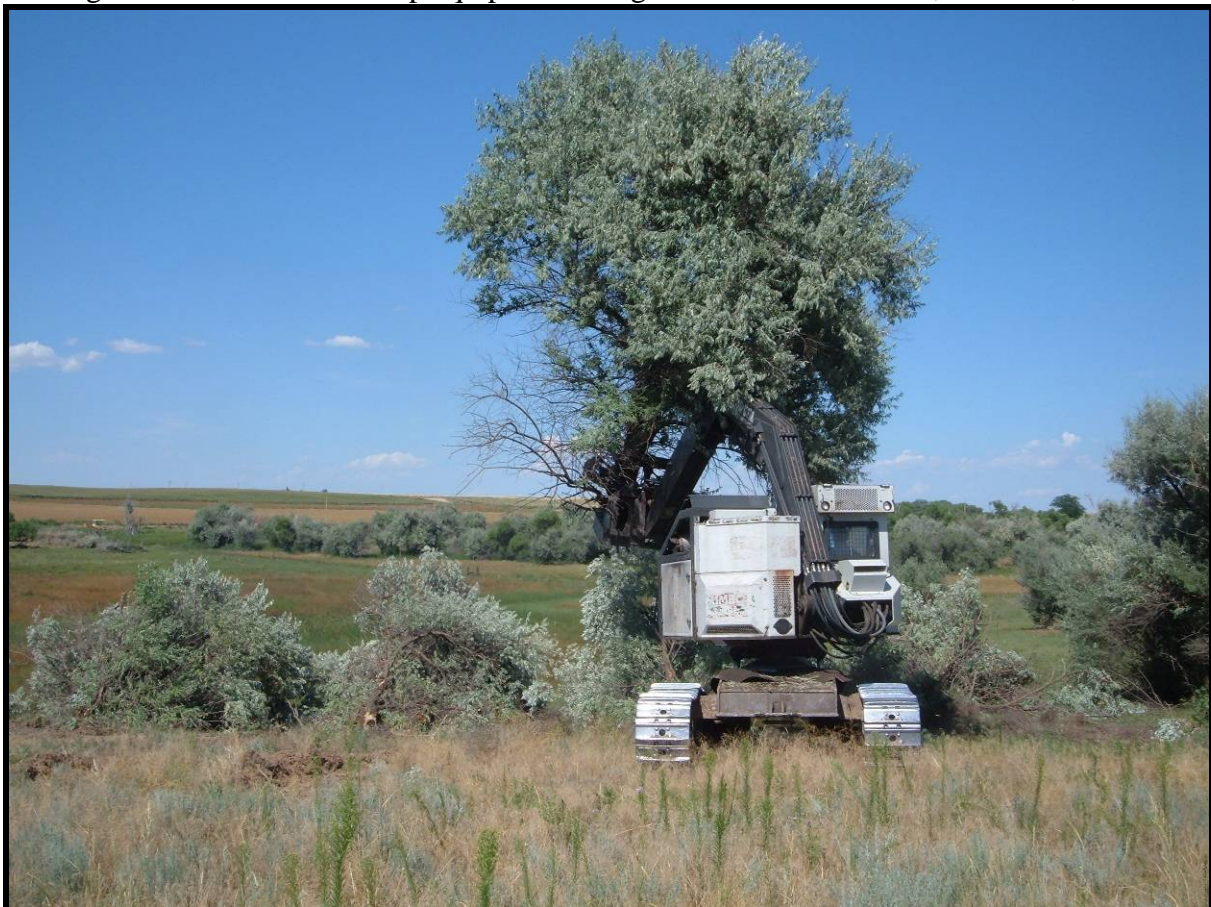
Figure 8: Grab & cut-stump equipment being used on 9-Mile Creek, Nebraska, 2004.
