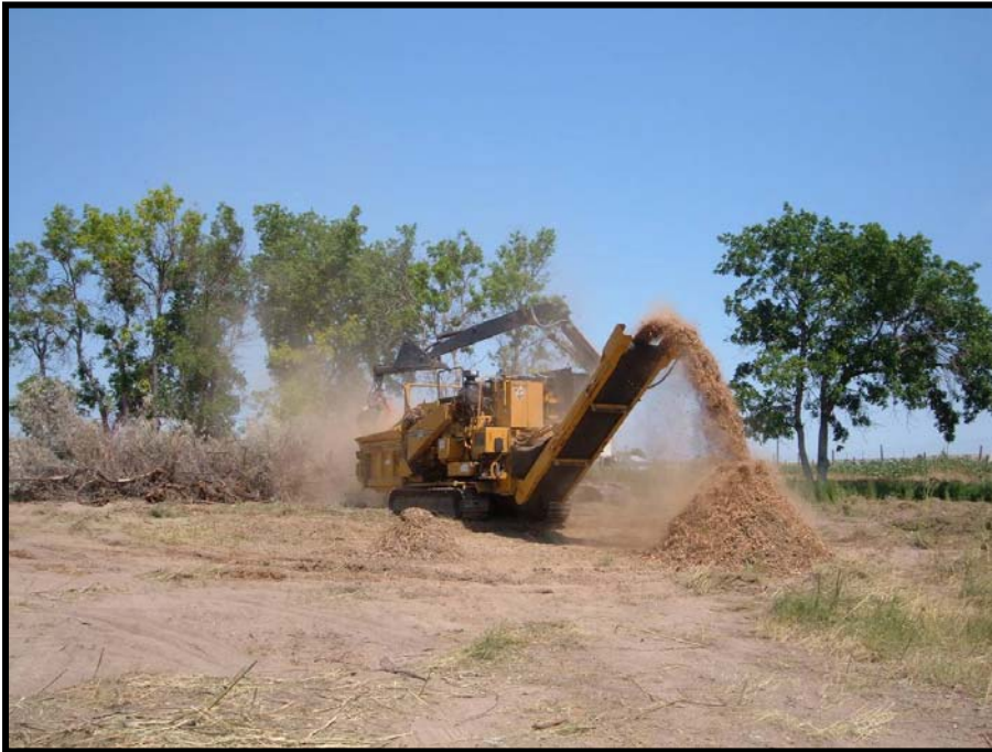
Figure 18: Large mobile chipper at work on 9-Mile Creek, Nebraska, 2004.
