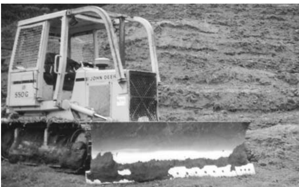
Bulldozers have been used to deep scalp the slopes for hand sowing.
