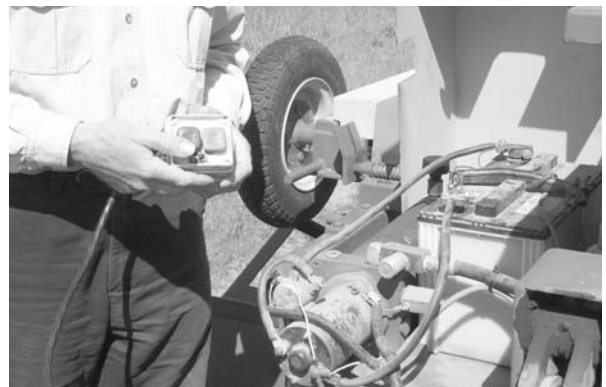
Hydraulics operated from cabin using battery powered motor
