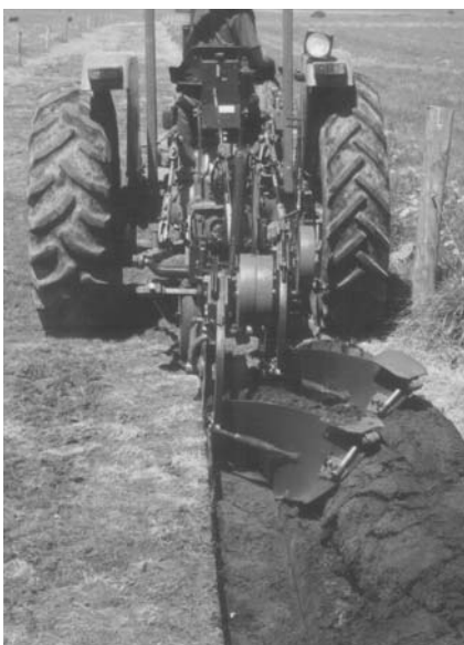
Mouldboard ploughing involves completely turning over the soil sod
