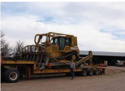
Ripper/Deep Chisel Type Root Plow
