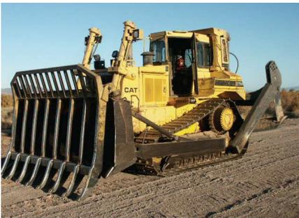
Ripper/Deep Chisel Type Root Plow
