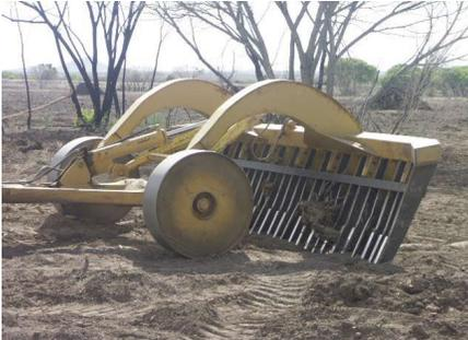
Ripper/Deep Chisel Type Root Plow
