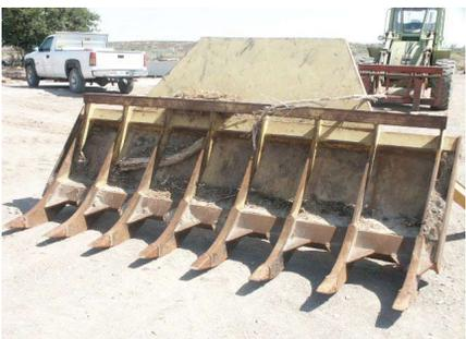
Ripper/Deep Chisel Type Root Plow
