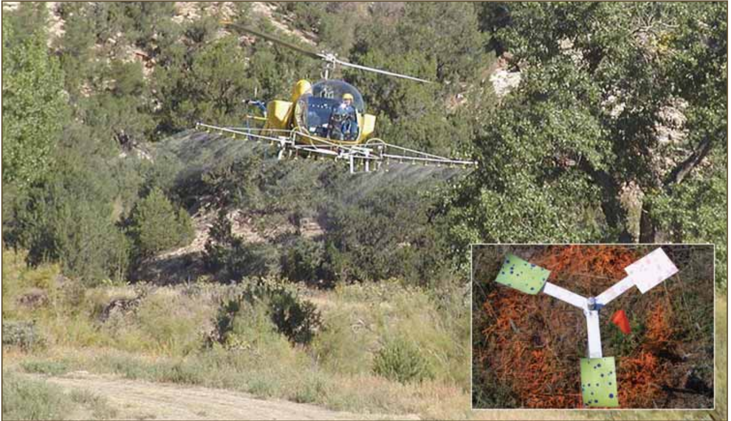
FIGURE 1. Helicopter making a 15 gallon/acre application and in this case avoiding a cottonwood tree. This helicopter carries about 70 gallons of spray solution. At 15 gallons/acre only 4 acres can be treated with a single load. The insert shows that the droplet size and spray pattern using water sensitive paper and an "artificial plant". This helicopter is operated by Olathe Spray Service, Inc., Olathe, CO. (Photos by J.R. Phillips)
