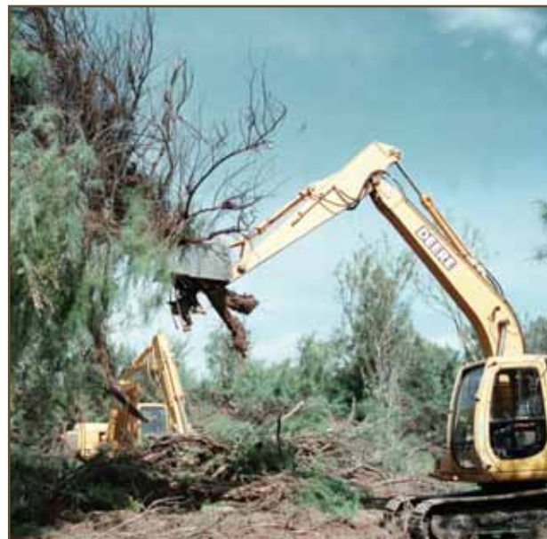
FIGURE 10. An example of individual tamarisk extraction using a track hoe. Notice that most of the crown has been removed. (Photo by Charlie Hart, Texas A&M)
